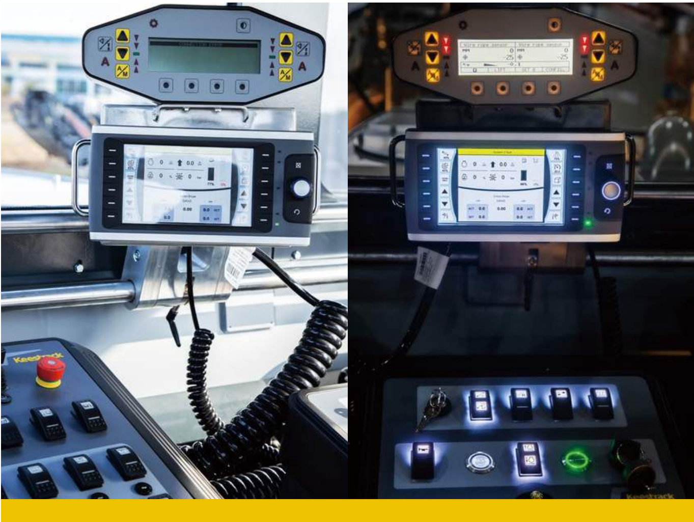
The control screen and MOBA panel are located within easy reach and in the operator's direct field of view
